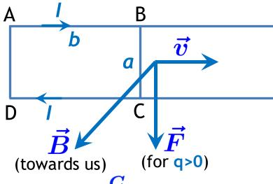
A fixed U-shaped loop; a crossbar (BC) moving with a speed v; uniform static external B-field.
