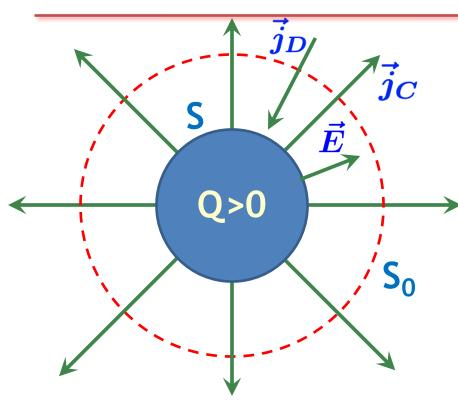
A charged sphere discharging into external conductive medium.
