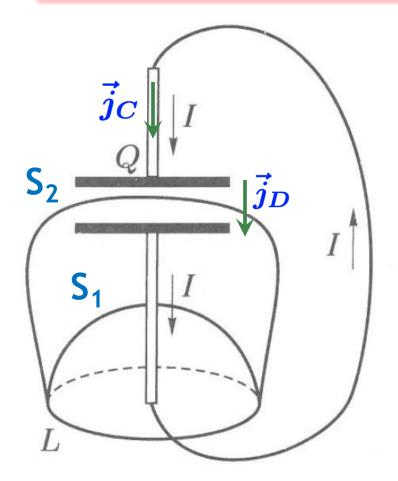
Discharge of a parallel-plate capacitor:
