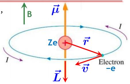
E-field induced in the electron orbit along the direction of motion:
