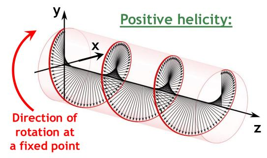
Elliptical polarisation: the field vector sweeps around an ellipse.
