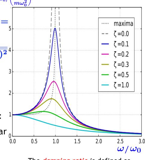
The *damping ratio* is defined as  $\xi = \gamma/(2\omega_0)$
