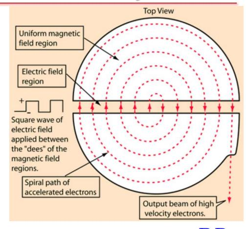
For elementary particles with q=e in magnetic field,  $p_{\perp}=eBR$  (in SI units)
