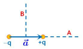
13) Consider a planar and a linear electric quadrupoles shown below. Using the definition of the dipole moment, check that the dipole moment of each system is zero. Find the direction and magnitude of the electric field on the axes of symmetry shown by the dashed lines, at a distance  $r \gg a$  from the centre of the quadrupole.
