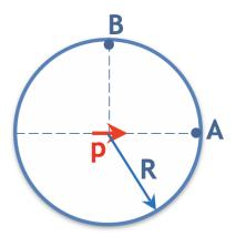
12) Consider a simple electric dipole consisting of two opposite point charges  $\pm q$  separated by a distance a. Using Coulomb's law, find the electrostatic potential  $\varphi$ , direction and magnitude of the electric field  $\vec{E}$  on the axis of the dipole (A) and in the plane of symmetry perpendicular to the axis (B) at a distance  $r \gg a$  from the dipole. Compare the results with those obtained in lecture 4 for the general case. Sketch the field lines.
