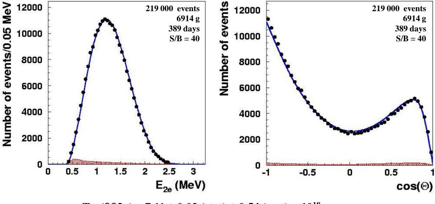
$T_{1/2}(\beta\beta 2\nu) = 7.11 \pm 0.02 \text{ (stat)} \pm 0.54 \text{ (syst)} \times 10^{18} \text{ years}$
