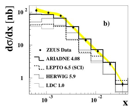
LEPTO, HERWIG (DGLAP) cannot reproduce the rates. LDC (based on CCFM evolution, linking DGLAP and BFKL) fails to describe data.
