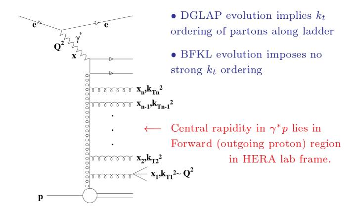
BFKL effects are expected to show up as enhanced high  $p_t$  particle production in the forward direction at HERA. Measurements are tricky, but there are many sensitive observables . . .
