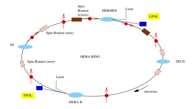
Spin rotators to be installed for H1 / ZEUS.
